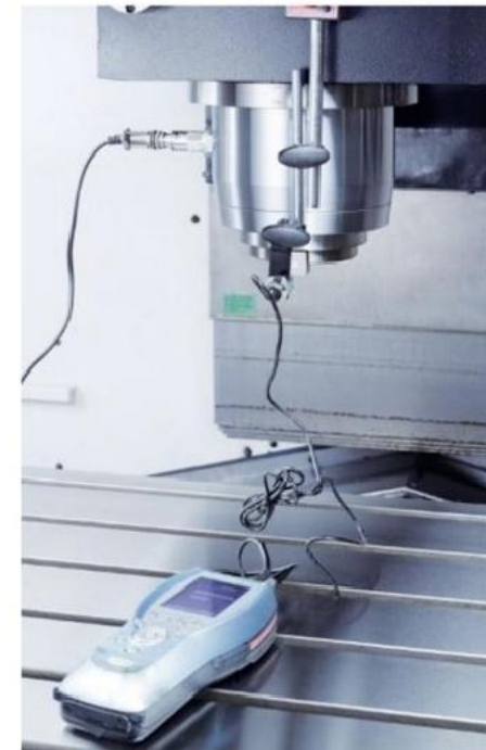
Renishaw QC 20 Ballbar System Used for detecting error-compensating movements of machine tools.
