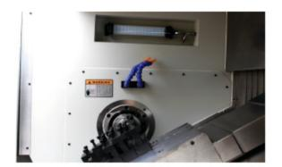
The fully enclosed casing design ensures the machine operator a clean and safe working environment.
